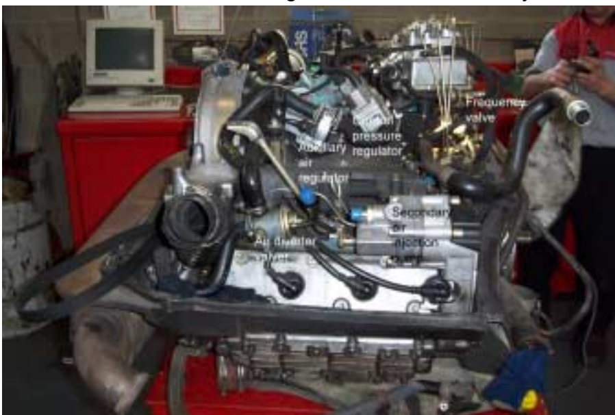
Air pump and secondary injection components. Photo by Kevin Ross
