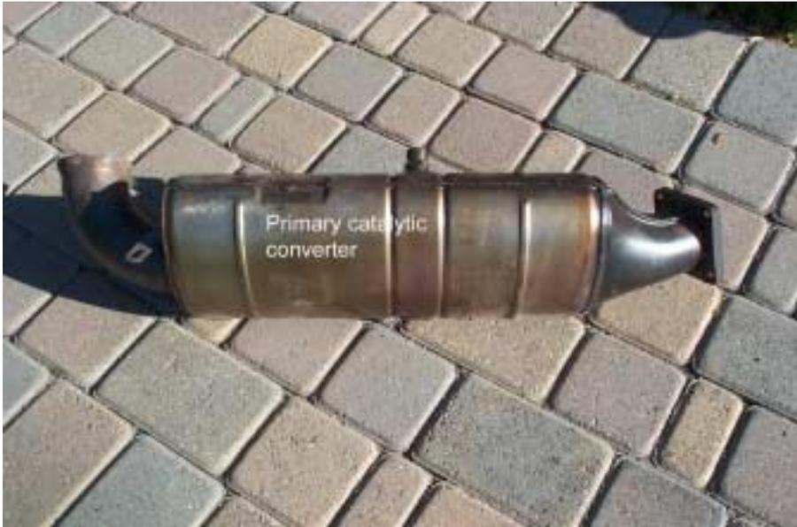
the catalytic converter are reduced approximately by this percentage. A catalytic converter has a limited life expectancy which depends upon use and external environmental conditions.
