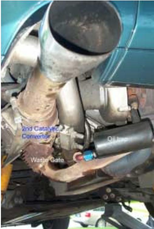
The left exhaust pipe is connected to the boost control valve (waste gate) and used to dump the excess boost pressure to the atmosphere. There is a secondary catalytic converter connected between the waste gate and the left hand exhaust tip. This is required because there is a direct input connection between the boost control valve and the exhaust system.
