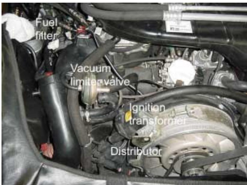
One ignition transformer with built in final driver stage. The ignition transformer is mounted above and to the right of the distributor assembly. Six spark plugs. Six spark plug lead set. A Bosch EZ69 electronic ignition control unit which is mounted to the right of the engine bay electrical distribution panel. The Ignition control unit relay (#1) is installed inside the engine bay electrical distribution panel.
