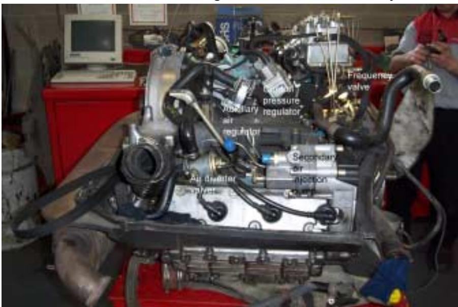
from flowing back through the system. If the engine is started with an engine oil temperature above 35° (95°F), the fresh air supplied by the secondary air pump is supplied to the catalytic converter, resulting in improved emission treatment.
